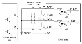
The control module is PNP type (common anode):
