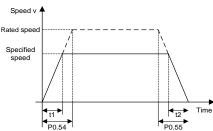
Note: ACC/DEC time can be used in the speed mode only.
