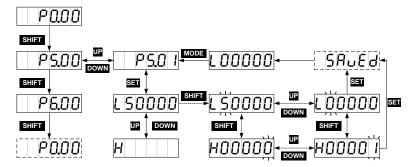
• Setting of long parameters (corresponds to parameters with over 6 digits) in parameter area:
