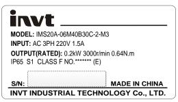
**Note:** "No.\*\*\*\*\*\*" in the nameplate is the motor model code (motor code for short). Please input this code into servo parameter P0.00 correctly (P0.00 is long parameter which can be set via keypad. See details at chapter 5.2.1 (8), otherwise, the servo system may not operate normally and major fault may occur to the drive and motor.
