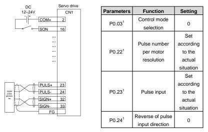
Step 1 Complete the connection between the drive and the servo motor.
