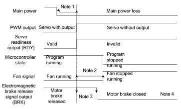
Note 1: If the voltage of the control power supply is less than 170V/330V(for 220V/400V series), the undervoltage fault will occur and the output level of the servo fault (ALM) will increase.
