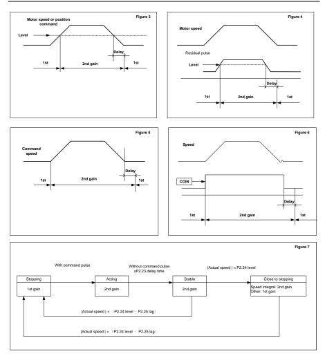
**Note:** The offset of gain switching sequence caused by lag (P2.25, P2.30, P2.34) is not reflected in above graphs.
