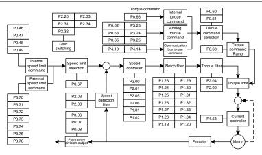
The common procedures for adjusting parameters in torque mode are as follows:
