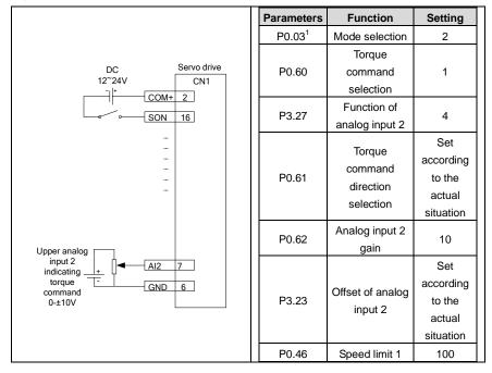
Step 1 Complete the connection between the drive and the servo motor.
