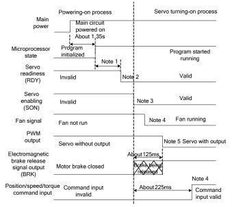
Note 1: The delay time from microprocessor initialization completion to servo readiness output can be set through P4.54.
