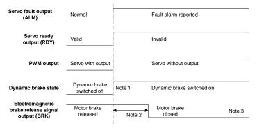
Note 1: Whether to immediately enable the dynamic brake can be set through P4.30. Note 2: The output delay of the electromagnetic brake release signal is specified by P3.57. If the speed slows down under the setting (30r/min by default) of P3.58 during the time specified by P3.57, the BRK signal becomes invalid.
