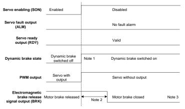
Note 1: Whether to immediately enable the dynamic brake can be set through P4.30. Note 2: The output delay of the electromagnetic brake release signal is specified by P3.57. If the speed slows down under the setting of P3.58 during the time specified by P3.57, the BRK signal becomes invalid.
